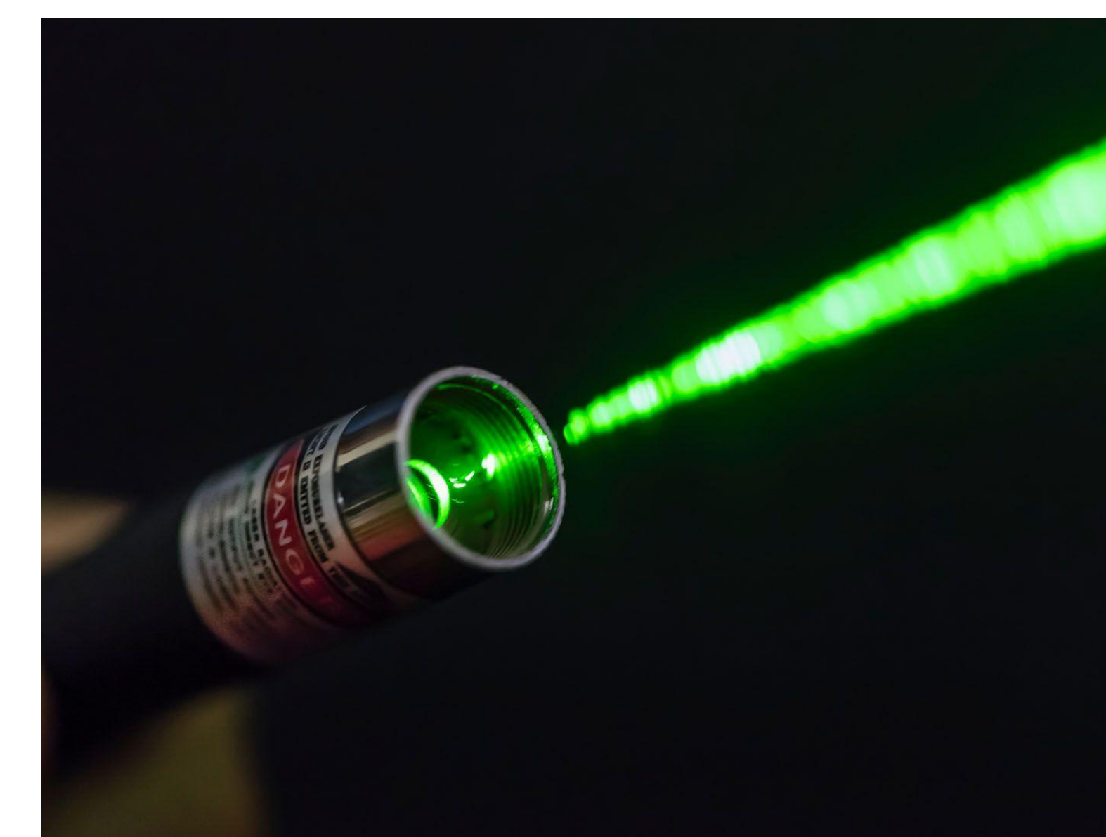
Figure 3. A green quantum well laser, which could be used in many of the applications listed below, including the observation of constellations in astronomy or other demonstrations.
