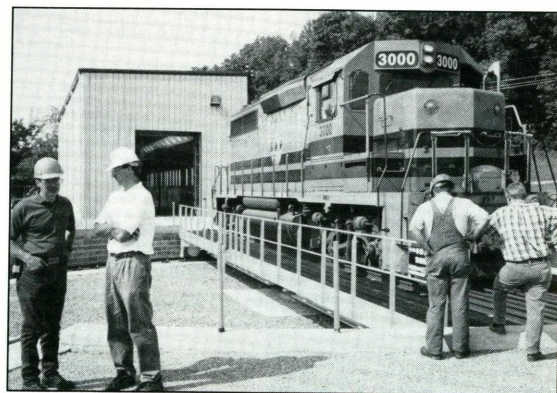
A 250-ton diesel electric locomotive rests on the turntable at Brookville Mining Equipment Corporation's new facility.
