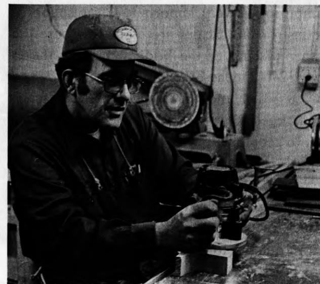
"My necks are made out of maple, birch, mahogany, or walnut. I cut the neck out and run the vibrator to get the shape I want. Then everything is glued together."
