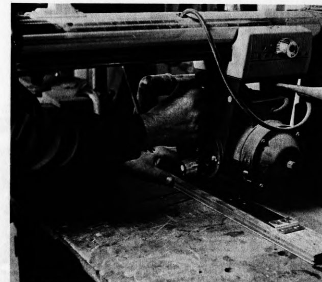
Using a jig to cut micarta
