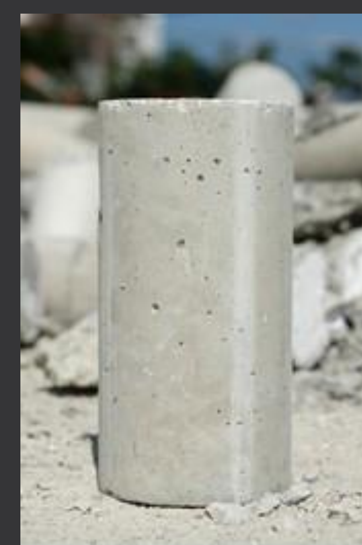
Figure 5. Concrete cylinder that would undergo compression testing
