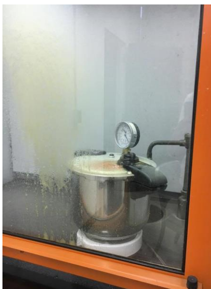
Figure 10: Result of yellow substance spewing from the release valve of the pressure cooker, coating the lid and fume hood sash in the substance.
