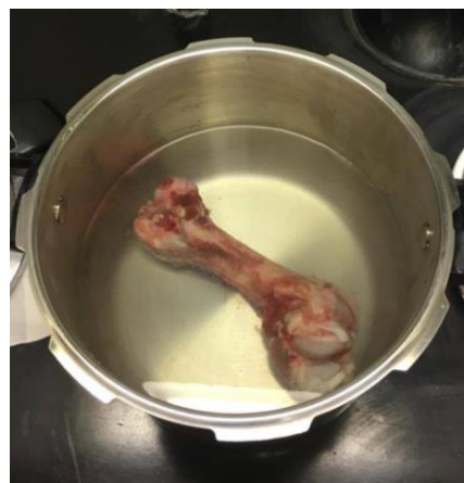
Figure 9: Placement of pig femur bone, filled halfway with 3.5 L KOH/H 2 O.
