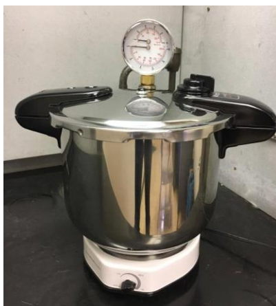
Figure 8: Pressure cookers set up with attached gauge and heating element.
