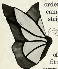
When each piece of glass has been fitted into its came, every “joint” is brushed with flux to insure a per-
