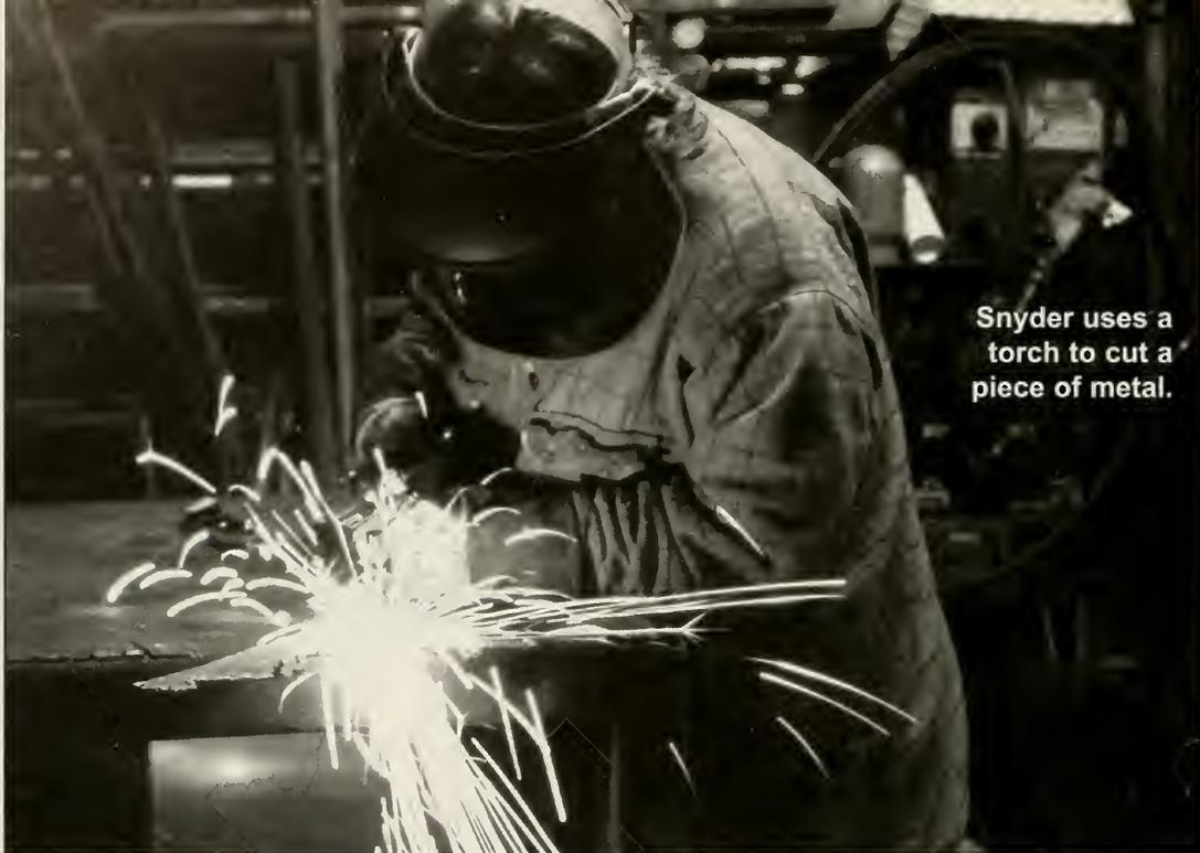
Snyder uses a torch to cut a piece of metal.
