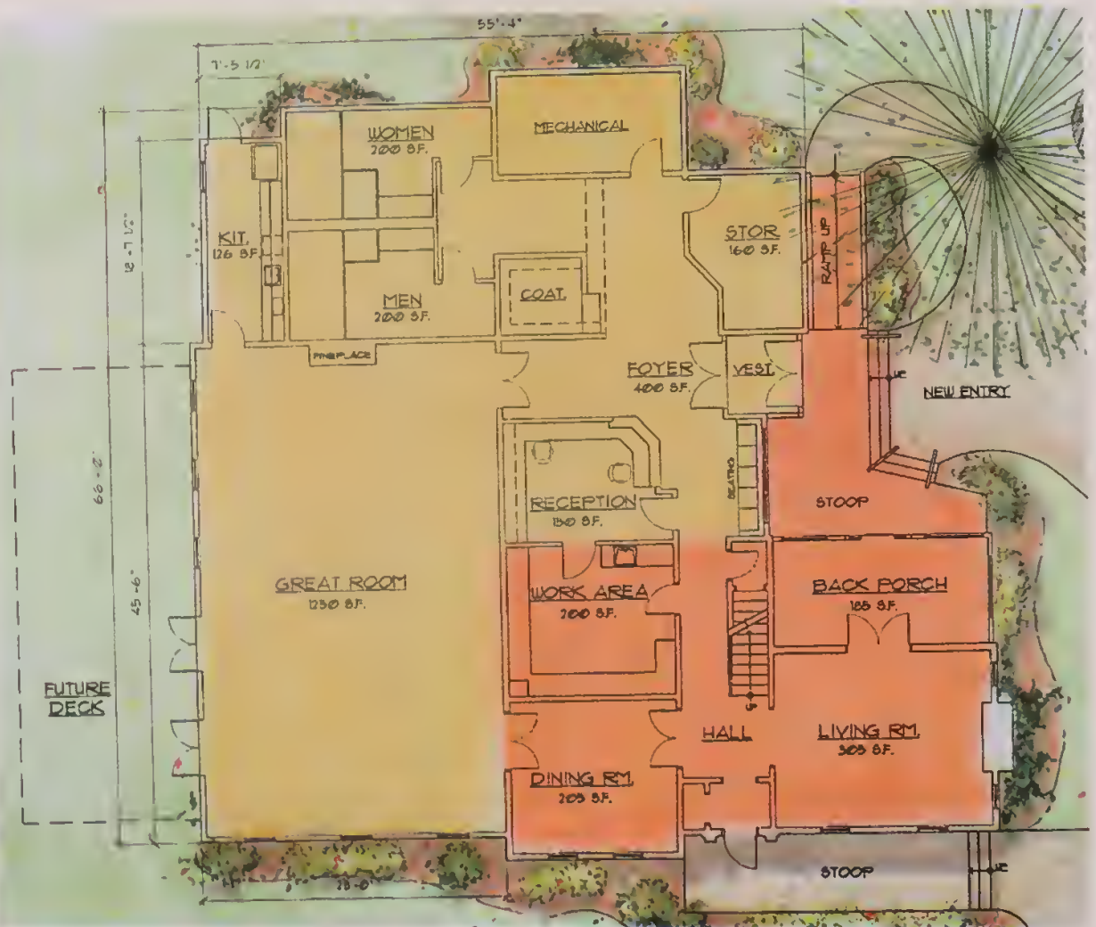
The existing Alumni House is shown in orange; the addition is shown in gold.
