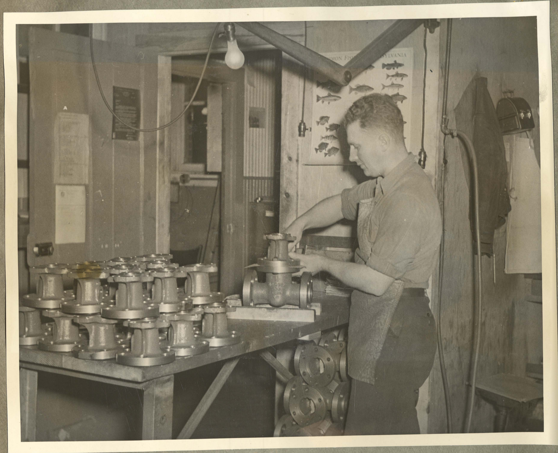
ASSEMBLING VALVES FOR SHIPMENT
