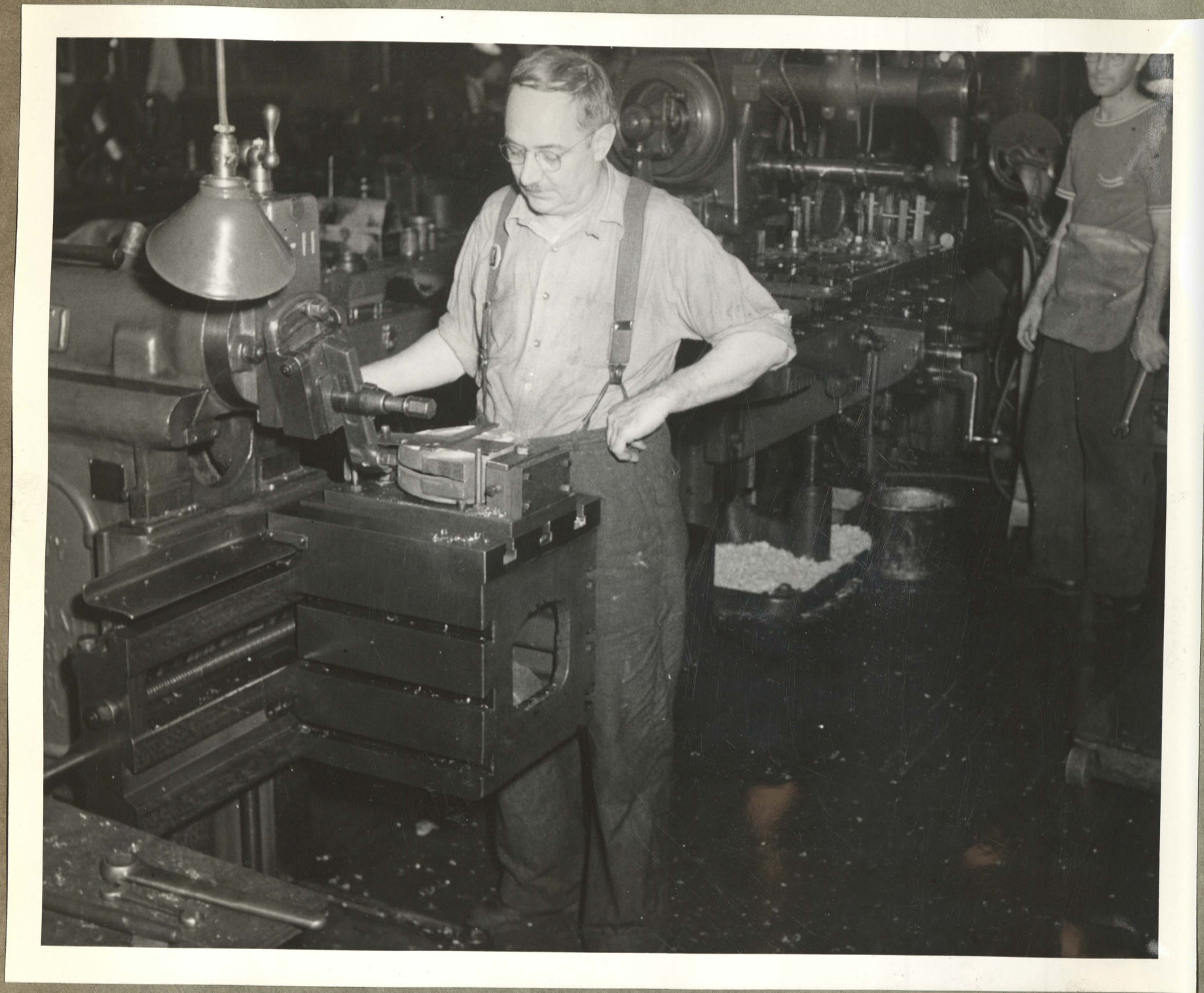
Shaper Operation on 6" Wedge
