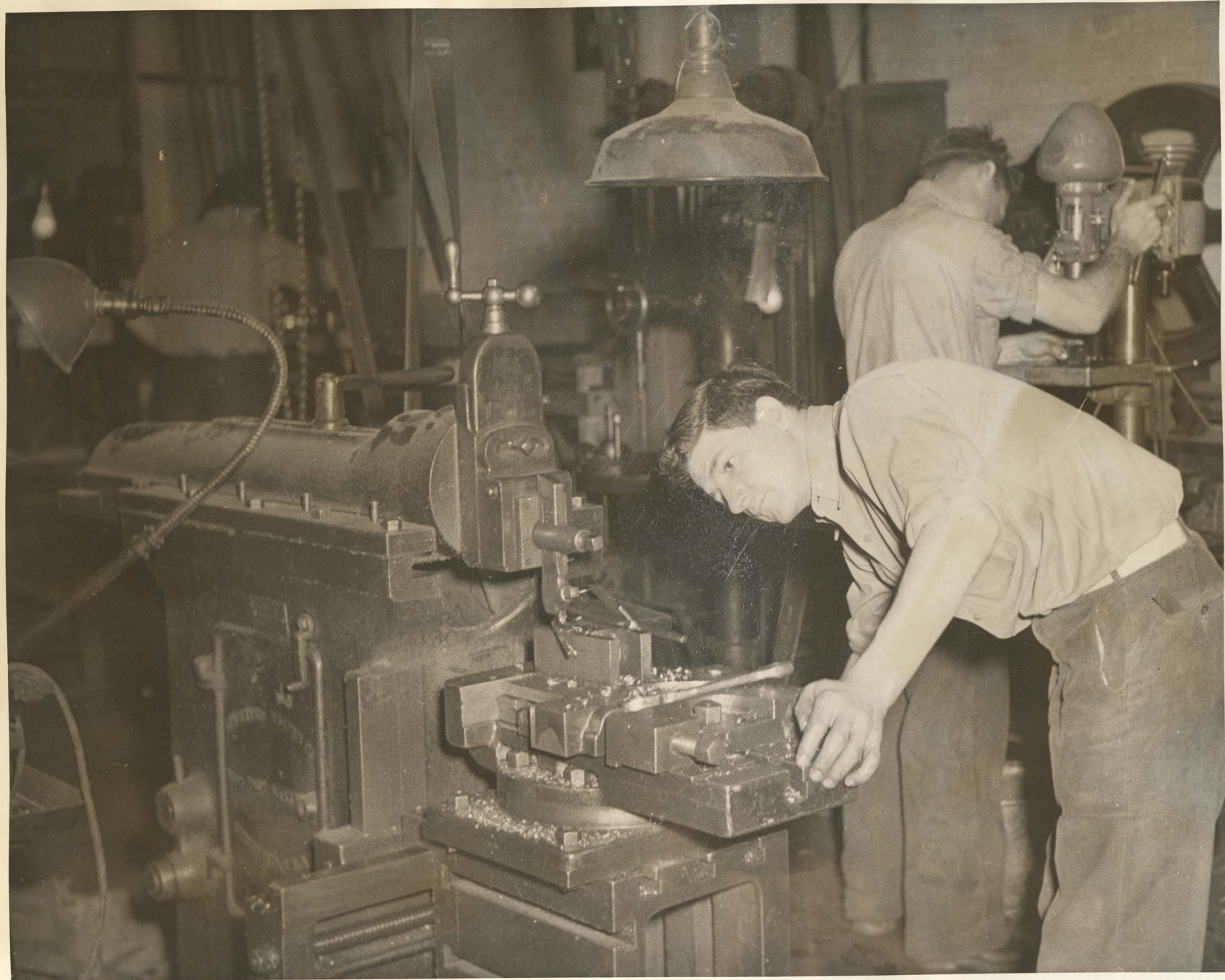
SHAPING GROOVES ON 1-1/2" WEDGE
