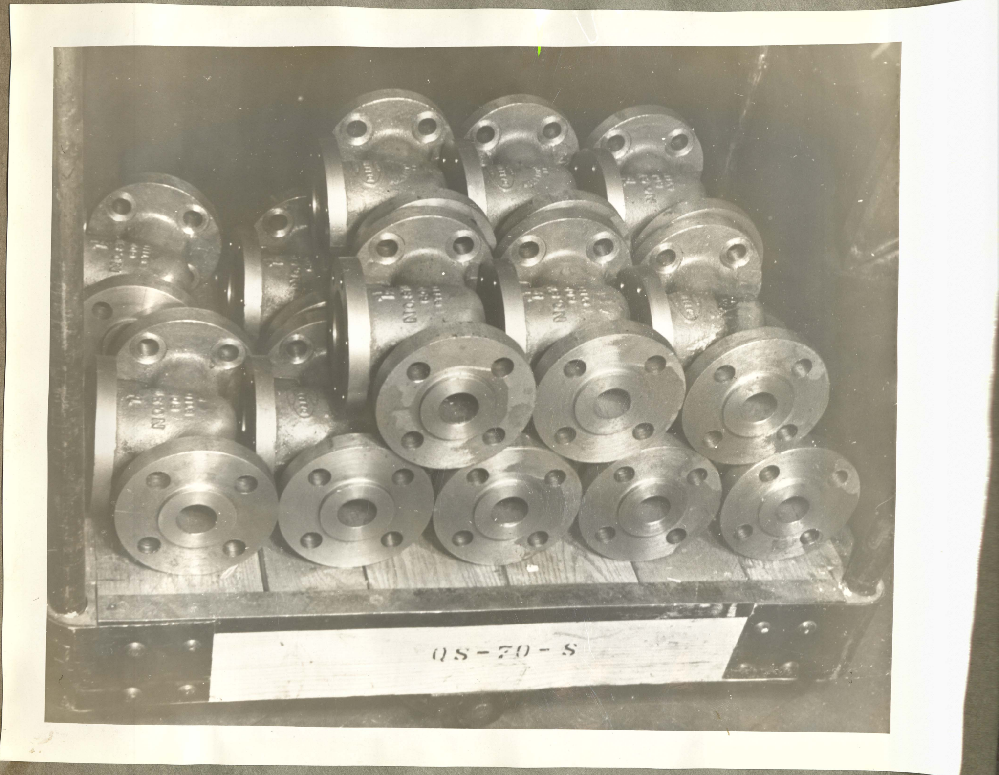
Finished 1-1/2" Valve Cases
