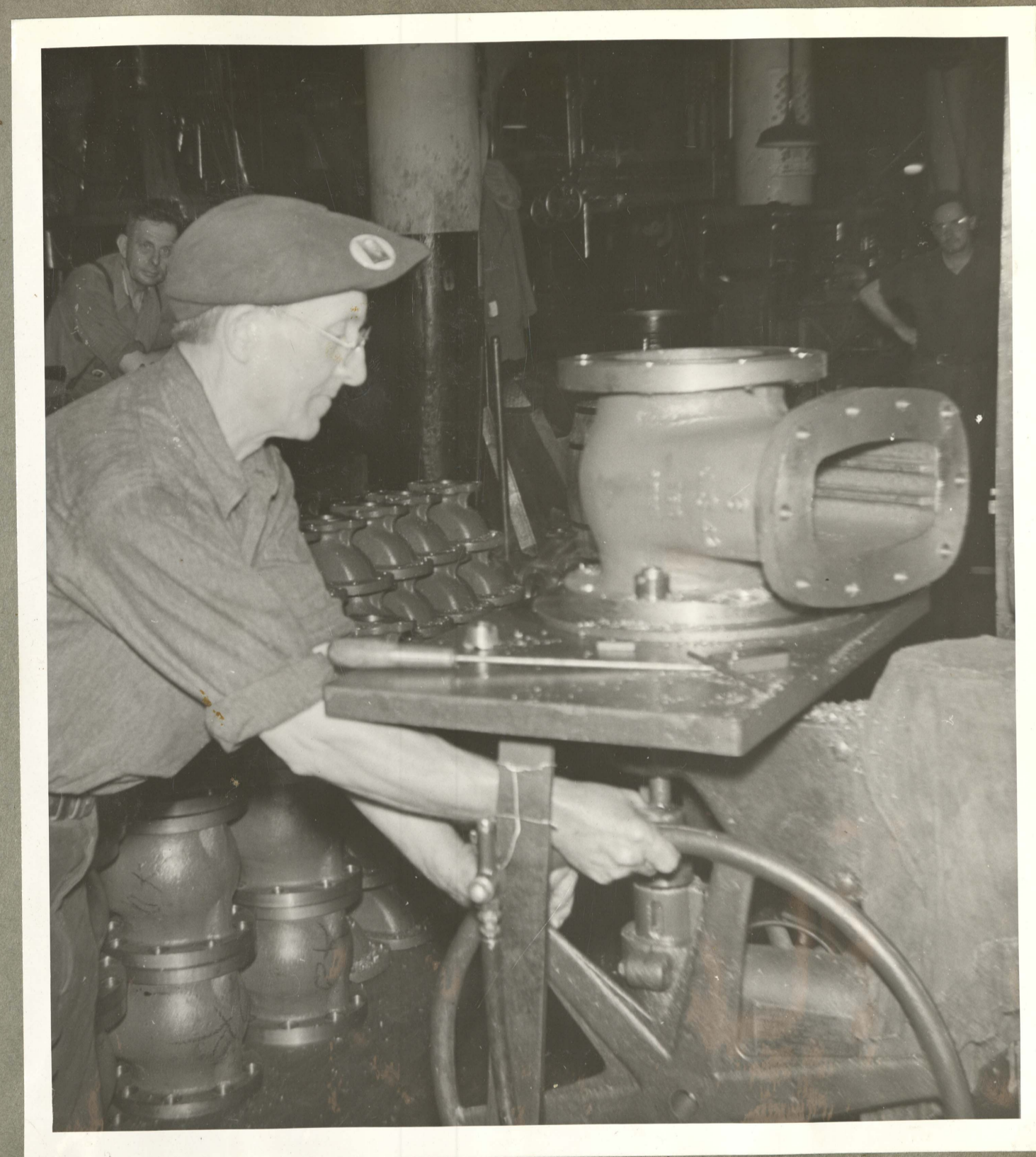
Spot Facing Holes in 6" Valve Case on Inverted Drill Press
