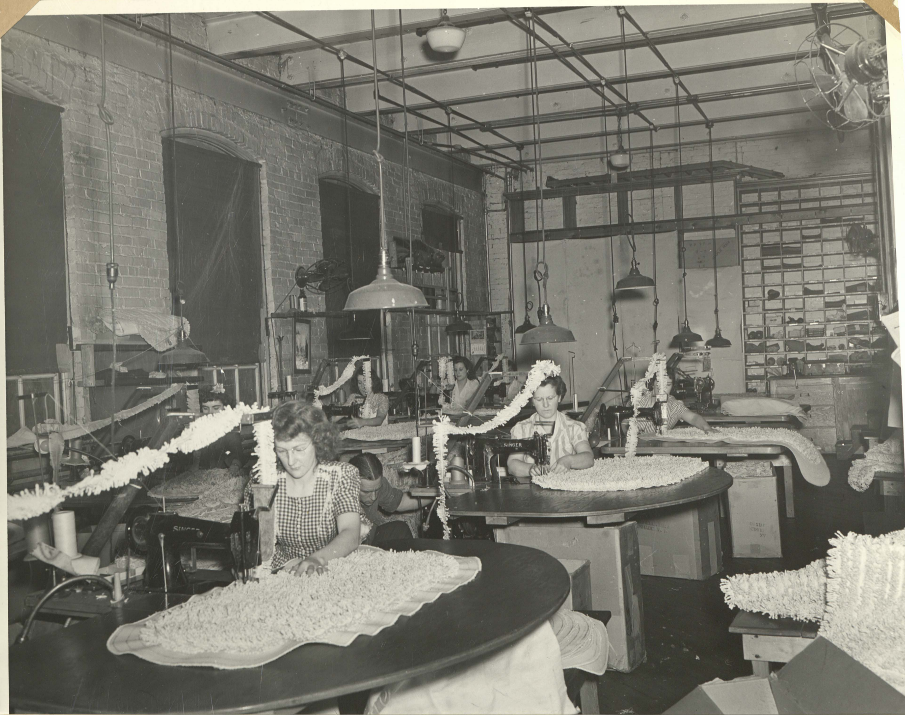
Sewing room of the cotton rug department of The Magee Carpet Company showing operators sewing fringe on duck backing. Building 3-2 1943 to the company by Brigadier General Allen R. Kimball.
