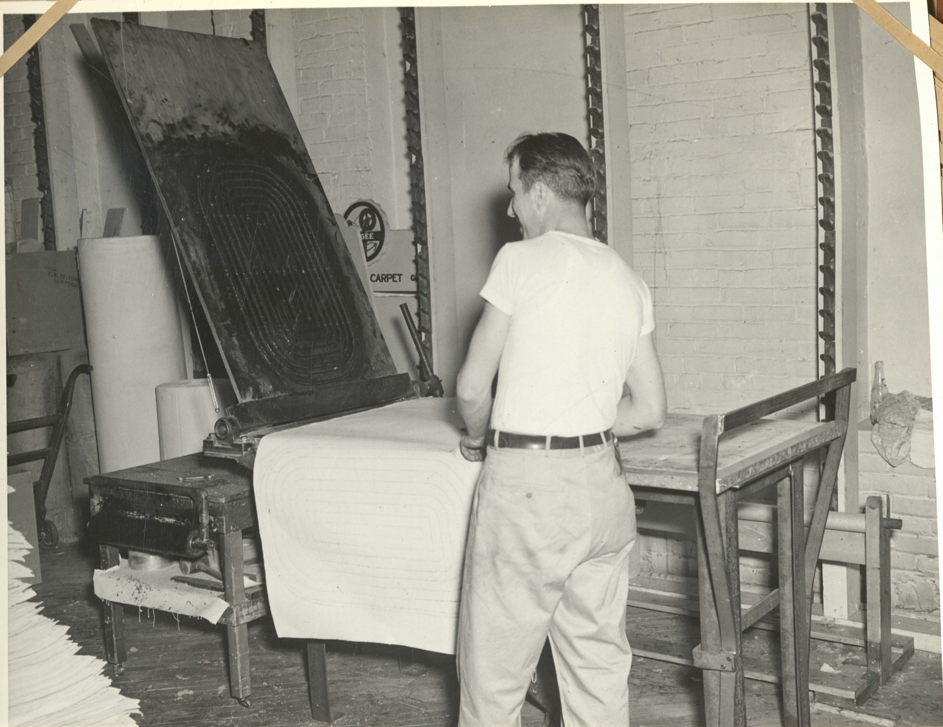
Printing machine used to mark guide lines on duck for sewing fringe of cotton rugs. Building 3-2 1943 Operator - Harold Keller
